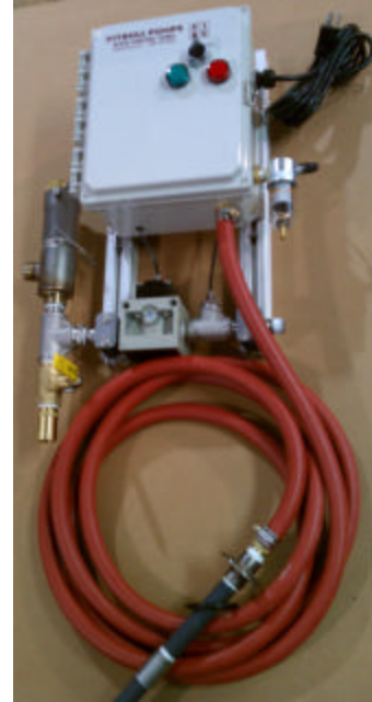
Control panel with probe and probe line.
