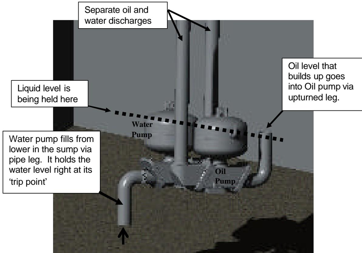
Oil coming into the sump will float on the surface in a layer that becomes thicker as it collects until it builds up to the 'oil' pump intake (just slightly above the 'dotted' operating level being held in the sump). From this condition forward, any oil coming into the sump carries over into the 'oil' pump intake and any water sinks and is picked up by the 'water' pump.
